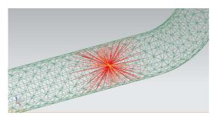
Fig. 4. RBE3 constraint of bushing contact area with bush stiffness
