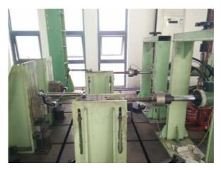
Fig. 10. Horizontal Fatigue MachineFig
