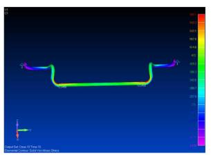
Fig. 7. Solid stressdistribution of RBE3 constraint
