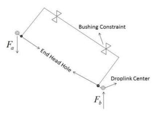
Fig. 2. The simplified forcediagramof the stabilizer bar
