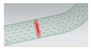
Fig. 3. The FEM of zero width RBE2 constrain
